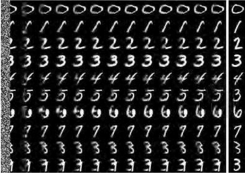
Figure 20.12: Illustration of clamping the right half of the image and running the Markov chain by resampling only the left half at each step. These samples come from a GSN trained to reconstruct MNIST digits at each time step using the walk-back procedure.
