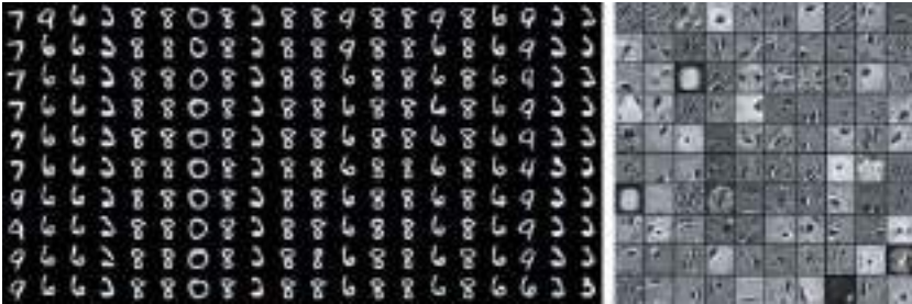
Figure 16.15: Samples from a trained RBM and its weights. ( Left ) Samples from a model trained on MNIST, drawn using Gibbs sampling. Each column is a separate Gibbs sampling process. Each row represents the output of another 1,000 steps of Gibbs sampling. Successive samples are highly correlated with one another. ( Right ) The corresponding weight vectors. Compare this to the samples and weights of a linear factor model, shown in figure 13.2. The samples here are much better because the RBM prior p(\mathbf{h}) is not constrained to be factorial. The RBM can learn which features should appear together when sampling. On the other hand, the RBM posterior p(\mathbf{h} \mid \mathbf{v}) is factorial, while the sparse coding posterior p(\mathbf{h} \mid \mathbf{v}) is not, so the sparse coding model may be better for feature extraction. Other models are able to have both a nonfactorial p(\mathbf{h}) and a nonfactorial p(\mathbf{h} \mid \mathbf{v}) . Image reproduced with permission from LISA (2008).
